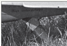
^ Undercarriage detail from 1481/18 showing an alternate tyre valve access hatch.
