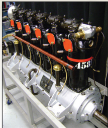
Unlike earlier versions of the Daimler-Mercedes D.III and D.IIIa, the engine numbers appear to have been regularly applied to D.IIIaü engines installed in the Pfalz D.XII and we have supplied decals [33], [34], [35] & [36] for you to choose from. The red bands [37] & [38] are not always clearly visible in archive photos but should be applied around every cylinder to indicate that they are over compressed.
