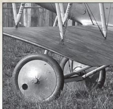
^ Undercarriage detail from 1491/18. Note the Pfalz factory logo 45 without additional 'D.XII' text on the fabric wheel cover.
