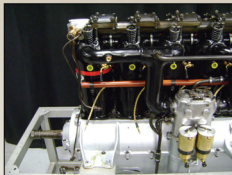
Water jacketed intake manifold and carburetor detail. A mount for the generator (943) can be seen at right but the actual generator was very rarely installed in fighter aircraft.
