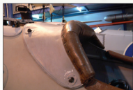
Aluminium cockpit coaming showing the method of stitching the padding. Note the turn buttons which attach the coaming to the fuselage.
