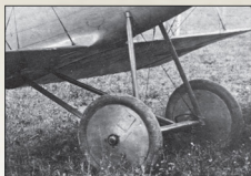
^ Undercarriage detail from 1481/18 showing an alternate tyre valve access hatch.
