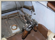
Hand air pump, fuel selector board and floor details. In service the fuel pipes were painted white with occasional red, yellow or blue rings (thanks Dan-San), oil pipes brown and air lines blue.
