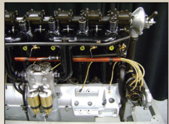
Water jacketed intake manifold and carburetor detail. A mount for the generator (943) can be seen at right but the actual generator was very rarely installed in fighter aircraft.
