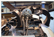
Twin LMG 08/15 'Spandau' mounts, ammunition feed chutes and twin flexible synchronizer cables for the guns.
